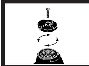
The deflector can be rotated to change the direction of the exhaust air. Disconnect air supply, loosen cap screw with a hex wrench, and then rotate deflector to desired direction. Tighten cap screw.
